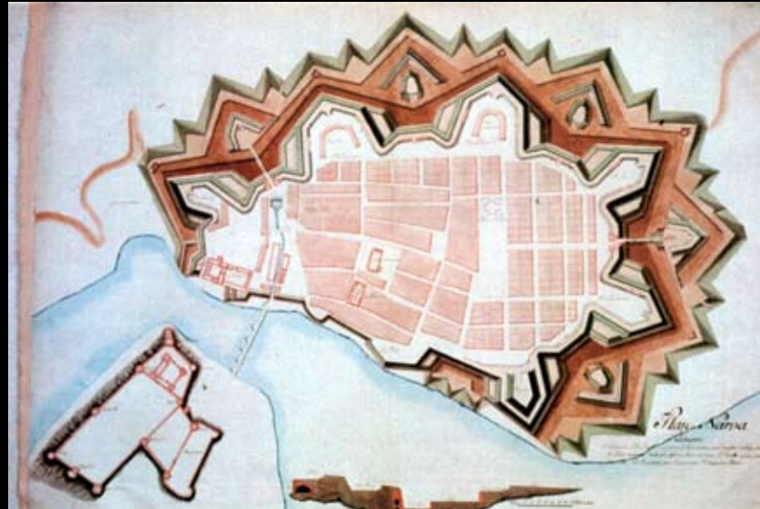
The project, devised by Erik Dahlberg in 1685, which became the basis for the construction of the bastions in Narva.
